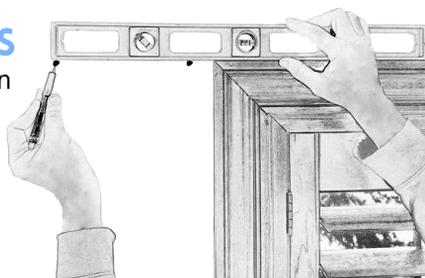
**TIP:** **Mounting height** depends on your curtain and hanging style. For example, curtains with grommets will hang higher than curtains with rings. There is also the option to puddle curtains on floor. We recommend getting a friend to help hold up your curtain with a rod section and fully assembled bracket to mark your desired height.
