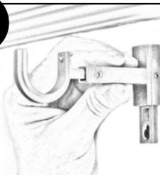
Ensure **2" vertical clearance** when mounting so brackets can slide over mounting plate. If no clearance, our brackets are designed to mount horizontally too. To mount horizontally remove cup from post and rotate cup upward.
