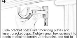
posts at desired length. At this point, add rod to check level. Slight adjustments can be made by moving mounting plates up or down if needed.
